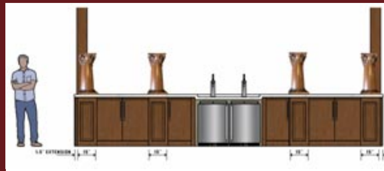
This schematic shows the new lower back bar being created to support the historic upper back bar. This is being custom built by the Wood Smiths cabinet makers of Kalamazoo, MI.
